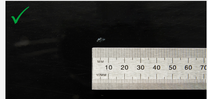
Dent less than 2mm deep and no wider than 20mm wide
